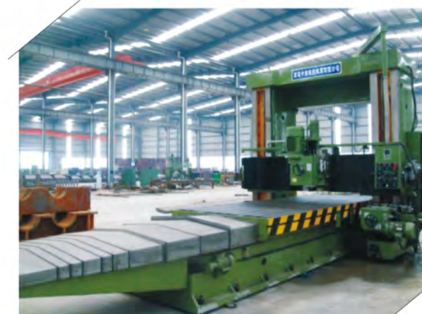
龙门铣床 Gantry Boring And Milling Machine
