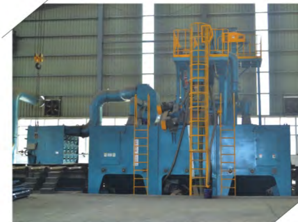
抛丸机 Shot Blasting Machine
