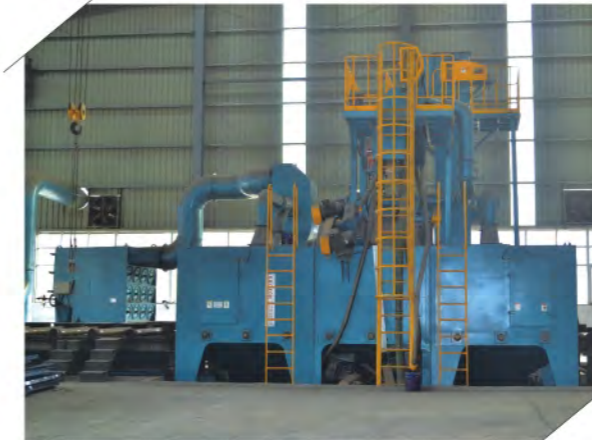
抛丸机 Shot Blasting Machine
