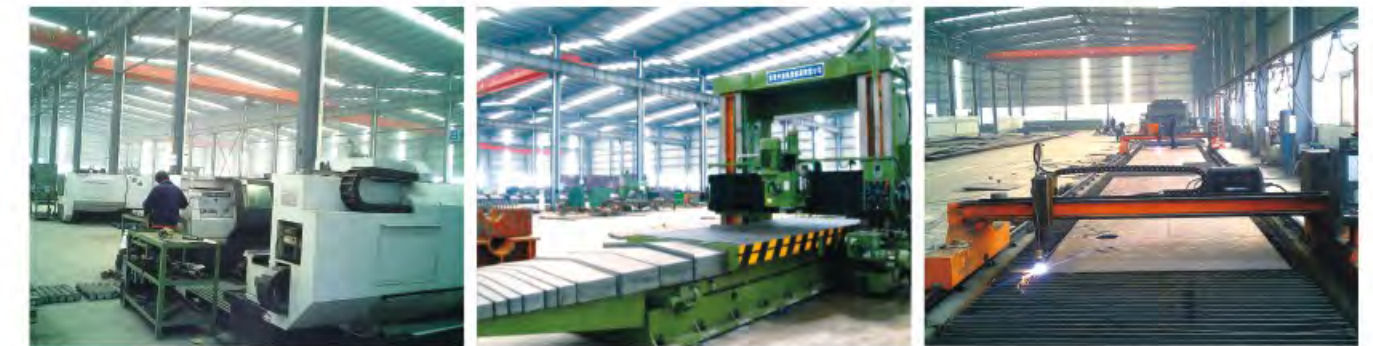
数控加工区 CNC Processing Area 龙门铣床 Gantry Boring And Milling Machine 数控等离子切割机 NC Plasma Cutting Machine
