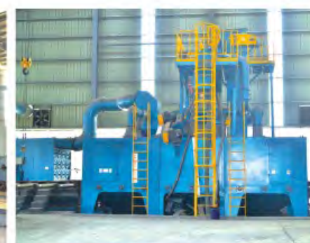
抛丸机 Shot Blasting Machine
