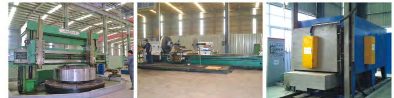
大型立车 Heavy Duty Vertical Lathe 大型卧式车床 Large Horizontal Lathe 大型热处理设备 Large-scale Heat Treatment Equipment
